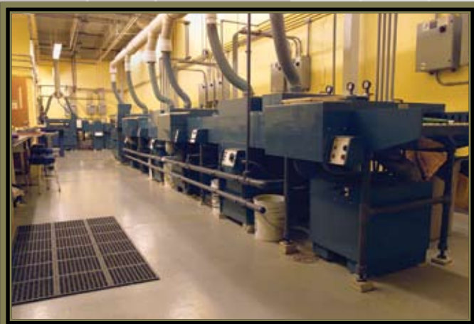
Etching: Metals are chemically etched in our etching lines where attention to the detail and intricacy of artwork is foremost. Ever concerned about the environment, our etching processes utilize a closed loop chemical treatment system that exceeds governmental requirements.
