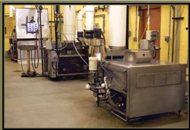
Crystal/Glass: Our “warm shop” consists of computer-controlled ovens in which we are able to heat crystal or glass to the stage where hand-cut pieces of glass actually become “fused” together. Through the use of molds crystal and glass can be “slumped” to make curved awards or shaped bowls.
