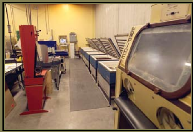
Crystal/Glass: Our “warm shop” consists of computer-controlled ovens in which we are able to heat crystal or glass to the stage where hand-cut pieces of glass actually become “fused” together. Through the use of molds crystal and glass can be “slumped” to make curved awards or shaped bowls.
